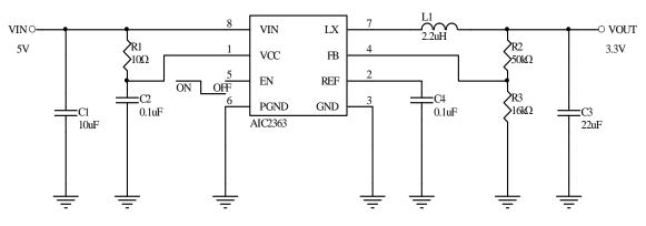
Fig. 2 Typical Application Circuit for SOP-8 Package
