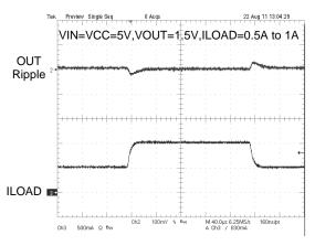
Fig. 10 Load Transient Response
