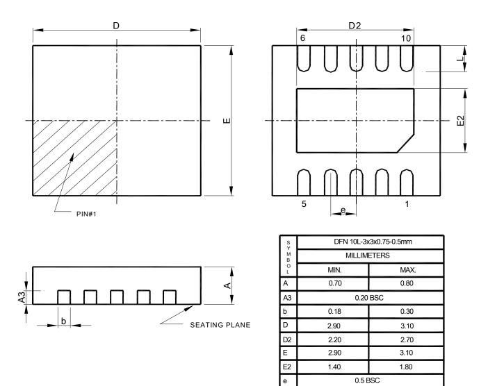
Note : 1. DIMENSION AND TOLERANCING CONFORM TO ASME Y14.5M-1994. 2.CONTROLLING DIMENSIONS : MILLIMETER , CONVERTED INCH DIMENSION ARE NOT NECESSARILY EXACT.
