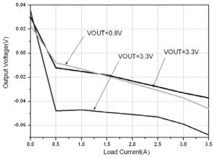
Fig. 12 Output Voltage Deviation vs Load Current
