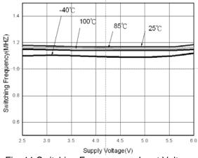
Fig. 11 Switching Frequence vs Input Voltage
